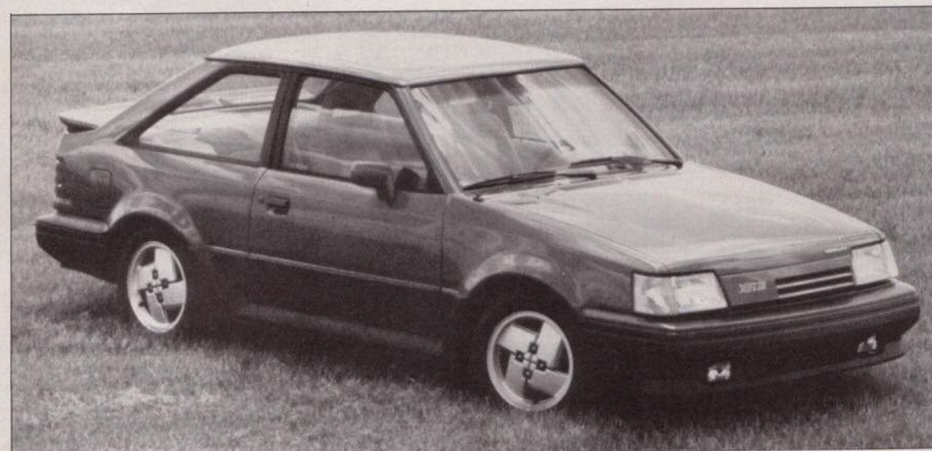
Mercury Lynx XR3 is a red-hot pocket rocket with the 115 hp, fuel-injected, 1.9-liter Four and 5-speed transmission.
