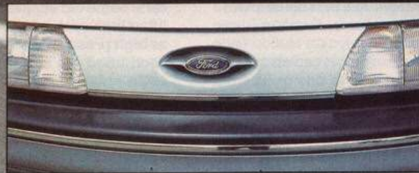
Aerodynamic touches on upscale Taurus nose include flush-fitting headlights, blocked-off grille with floating Ford logo.
