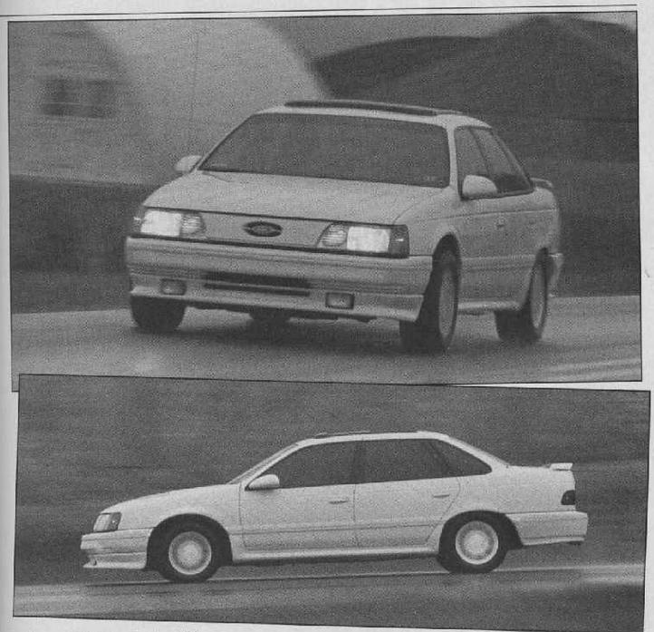
braking or spirited cornering. In addition, the stiff springs, in combination with the wide tires, frustrate the linear steering and the comfortable ride of the stock Taurus. The JMX Taurus undoubtedly has more grip than the stock car, thanks to its stickier rubber and lower ride height, but the smoothness and precision of the factory scup are gone. If you value refined hardling, don't fix what isn't broken.
